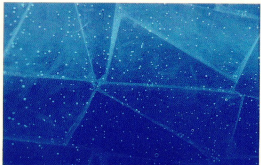
Fig. 15. A natural opal mosaic triplet under long-wave ultraviolet radiation. Note the fluorescence of the adhesive between the opal sections. Under this magnification phosphorescence is seen to come from the opal sections and not the adhesive - the reverse was the case for the Opalite mosaic triplets. Photo by John I. Koivula.
